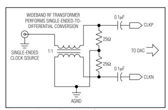
Figure 4. Differential Clock-Signal Generation
