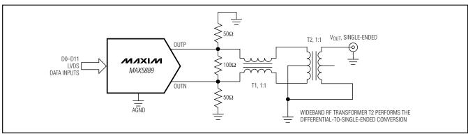
Figure 5. Differential-to-Single-Ended Conversion Using a Wideband RF Transformer
