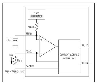
Figure 1. Reference Architecture, Internal Reference Configuration
