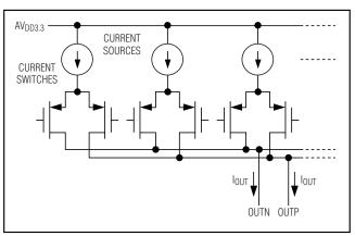
Figure 2. Simplified Analog Output Structure
