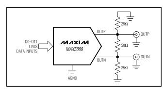
Figure 6. Differential Output Configuration
