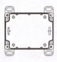
Feet can be mounted in either direction
