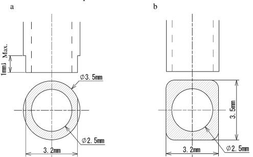
\*Nozzle with chamfering is recommended
