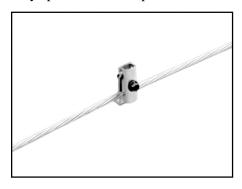
4.3 Tighten bolt in external bonding/hanger bracket to approximately 50 inch pounds (565 cm • N) to secure hanger. For self-supporting cable tighten to 75 inch pounds (850 cm • N) to secure hanger.
