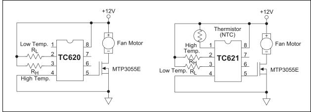
FIGURE 4-2: Temperature Controlled Fan.
