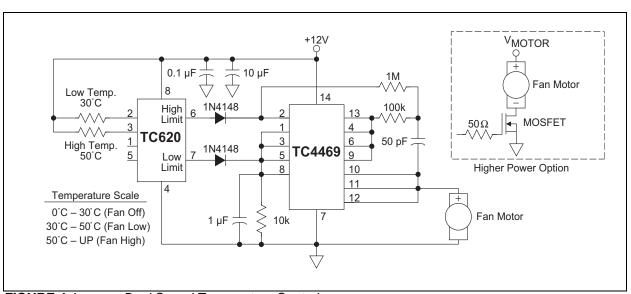
FIGURE 4-1: Dual Speed Temperature Control.
