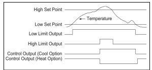
**FIGURE 3-1:** TC620/TC621 Input vs. Output Logic.
