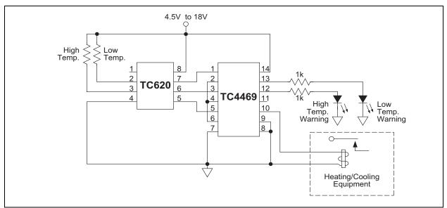
FIGURE 4-3: Heating and Cooling Application.
