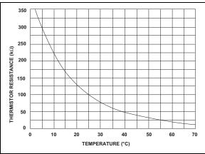
FIGURE 3-4: Typical NTC Thermistor.
