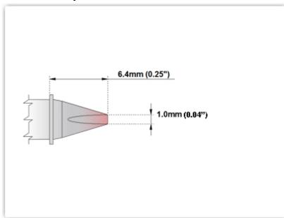
EPM75CH179 Chisel 30° 1.0mm (0.04")
