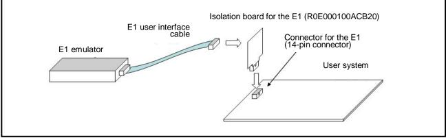
Figure 4.1 Mounting the R0E000010ACB20
