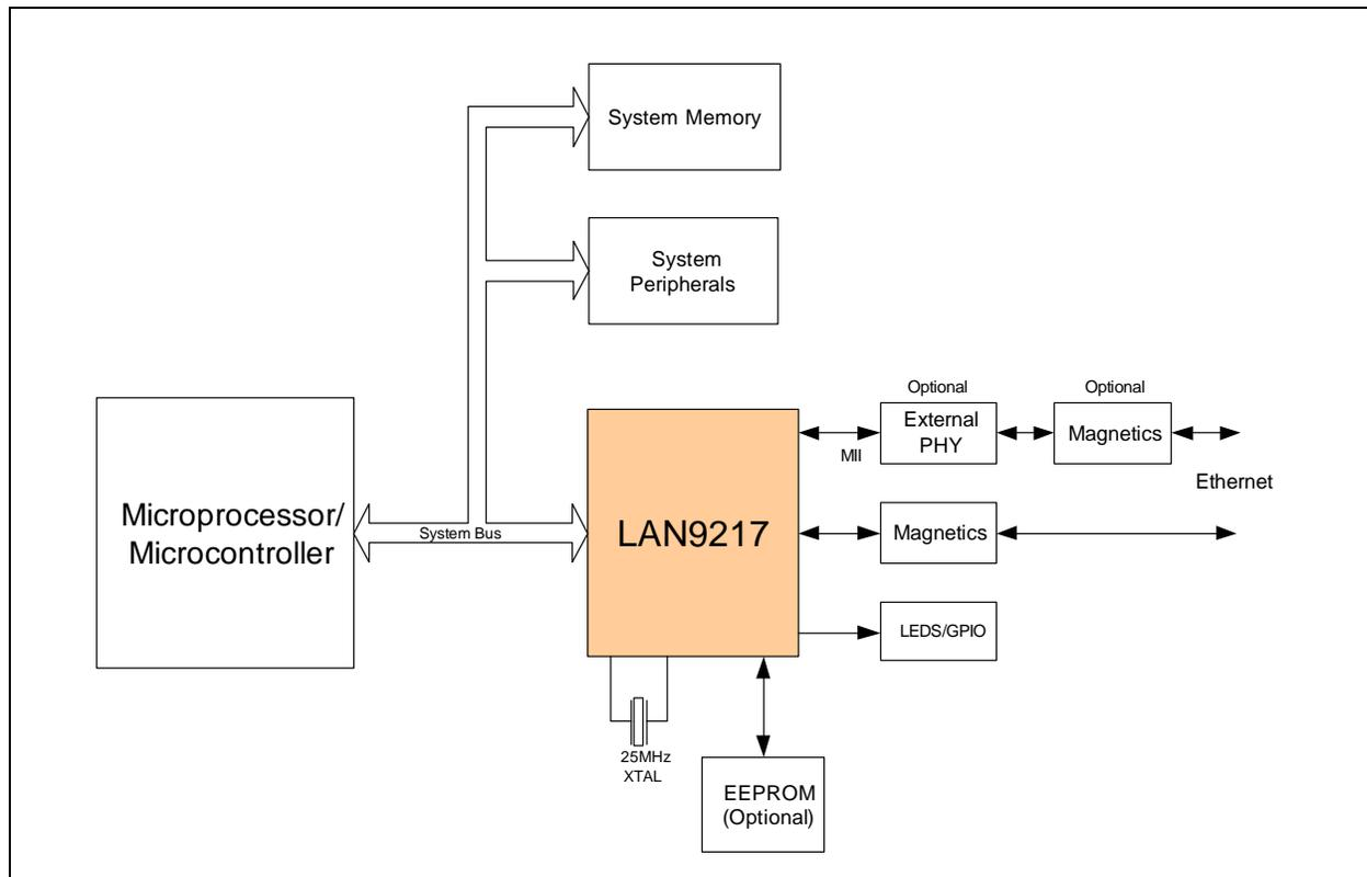
The Microchip LAN9217 integrated 10/100 MAC/PHY controller is a peripheral chip that performs the function of translating parallel data from a host controller into Ethernet packets. The LAN9217 Ethernet MAC/PHY controller is designed and optimized to function in an embedded environment. All communication is performed with programmed I/O transactions using the simple SRAM-like host interface bus.
