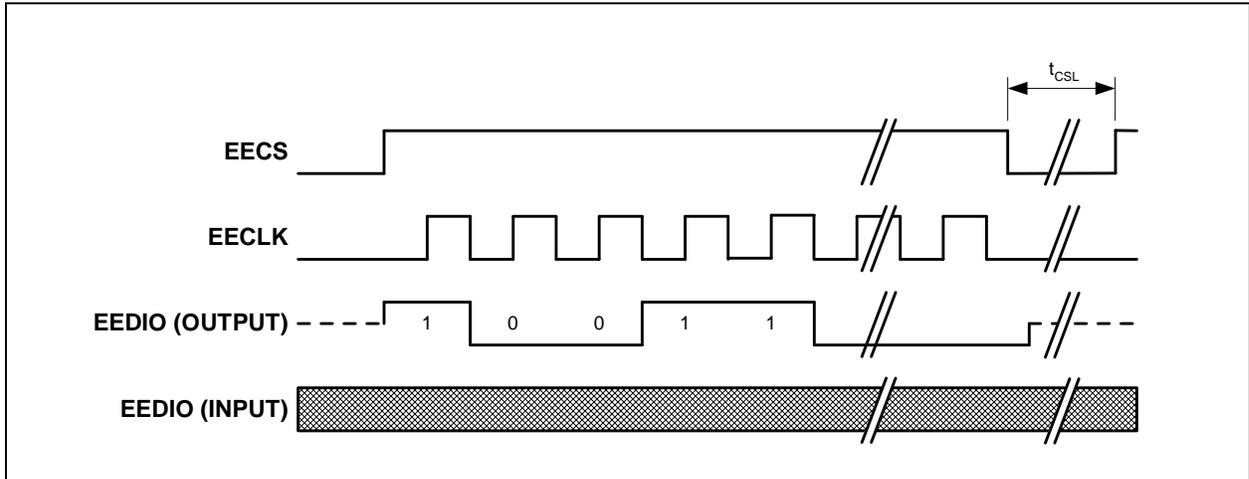
**READ (Read Location):** This command will cause a read of the EEPROM location pointed to by EPC Address (EPC\_ADDR). The result of the read is available in the E2P\_DATA register.
