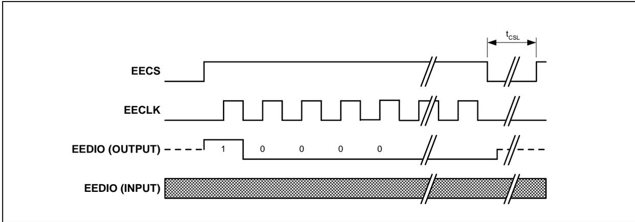
**EWEN (Erase/Write Enable):** Enables the EEPROM for erase and write operations. The EEPROM will allow erase and write operations until the “Erase/Write Disable” command is sent, or until power is cycled.
