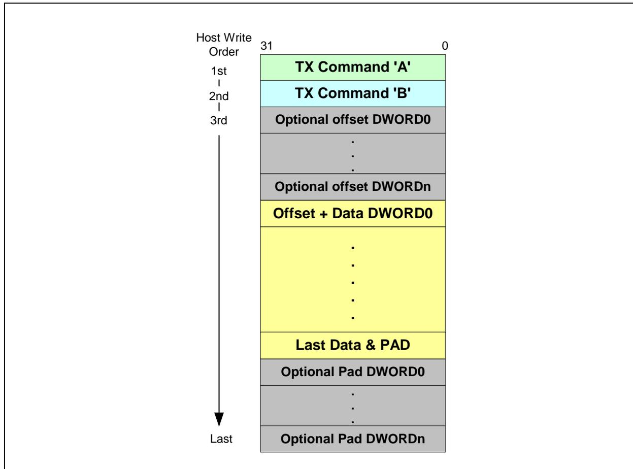
Figure 3-13, "TX Buffer Format", shows the TX Buffer as it is written into the LAN9217. It should be noted that not all of the data shown in this diagram is actually stored in the TX data FIFO. This must be taken into account when calculating the actual TX data FIFO usage. Please refer to [Section 3.12.5, "Calculating Actual TX Data FIFO Usage," on page 45](#) for a detailed explanation on calculating the actual TX data FIFO usage.
