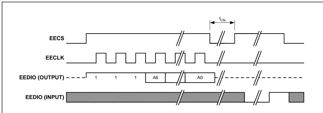
**ERAL (Erase All):** If erase/write operations are enabled in the EEPROM, this command will initiate a bulk erase of the entire EEPROM. The EPC\_TO bit is set if the EEPROM does not respond within 30ms.
