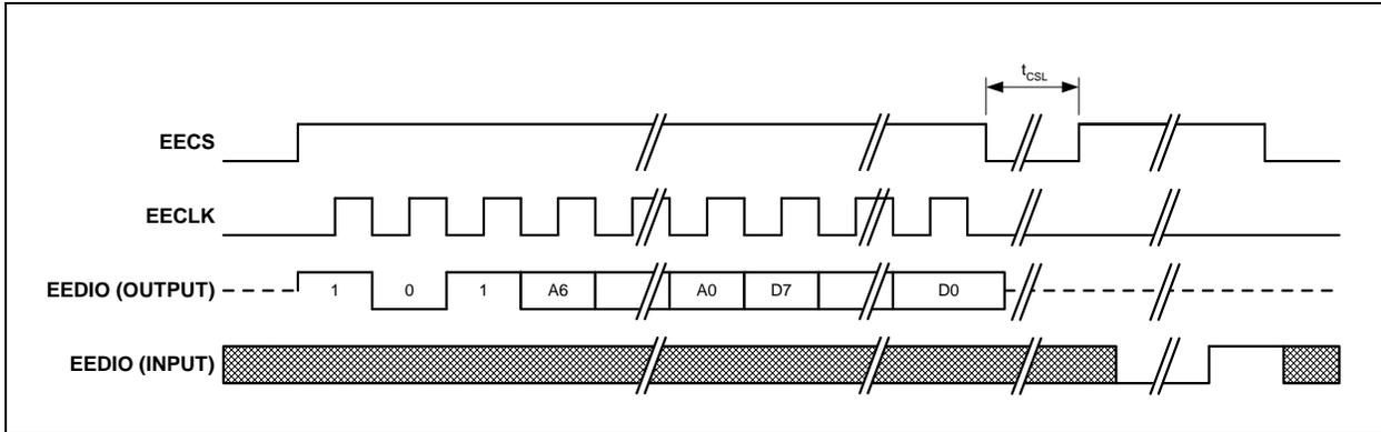
**WRAL (Write All):** If erase/write operations are enabled in the EEPROM, this command will cause the contents of the E2P\_DATA register to be written to every EEPROM memory location. The EPC\_TO bit is set if the EEPROM does not respond within 30ms.
