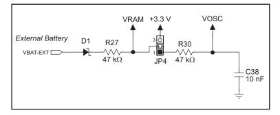
Figure C-2. RCM4000 Backup Battery Circuit
