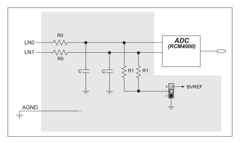
Figure 10. Resistor Divider Network for Analog Inputs
