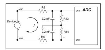
Figure 11. Current Flow from Ungrounded or Floating Source
