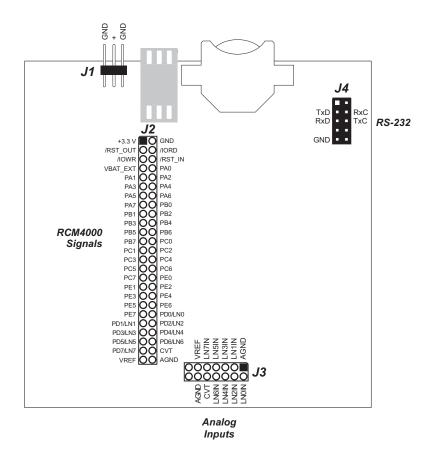
Figure B-4. Prototyping Board Pinout
