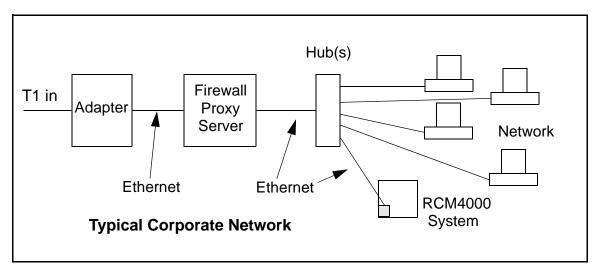
If your system administrator can give you an Ethernet cable along with its IP address, the netmask and the gateway address, then you may be able to run the sample programs without having to setup a direct connection between your computer and the RCM4000. You will also need the IP address of the nameserver, the name or IP address of your mail server, and your domain name for some of the sample programs.
