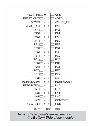
Figure 6. RCM4000 Pinout
