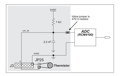
Figure B-7. Prototyping Board Thermistor Input
