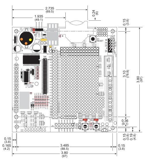
Figure B-2. Prototyping Board Dimensions
