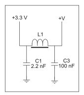
Figure 13. Analog Supply Circuit
