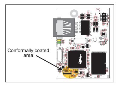
Figure A-5. RCM4000 Areas Receiving Conformal Coating
