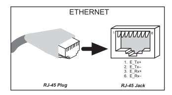
Figure 8. RJ-45 Ethernet Port Pinout
