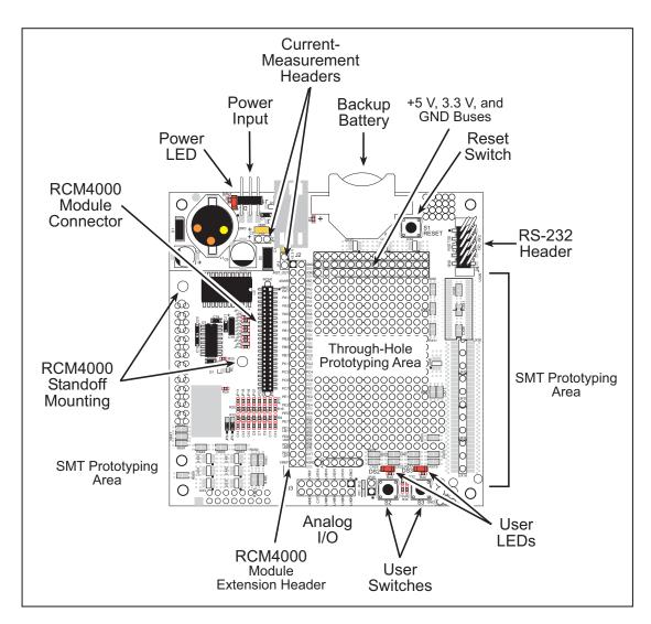
The Prototyping Board is shown below in Figure B-1, with its main features identified.
