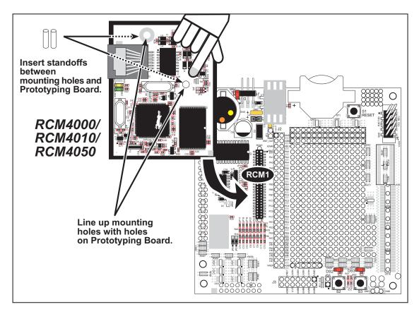
Figure 3. Install the Module on the Prototyping Board
