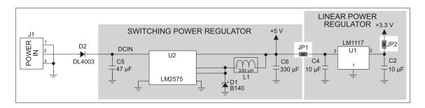
Figure B-3. Prototyping Board Power Supply
