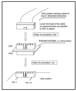
Figure 2 Usage of the R0E000010ACB00
