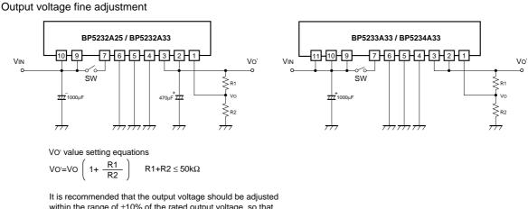
It is recommended that the output voltage should be adjusted within the range of  $\pm 10\%$  of the rated output voltage, so that the performance of the module can fully be exhibited.
