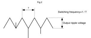
Note that the output ripple voltage depends on the type and characteristics of the output capacitor.
