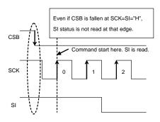
Figure 43. Operating timing
