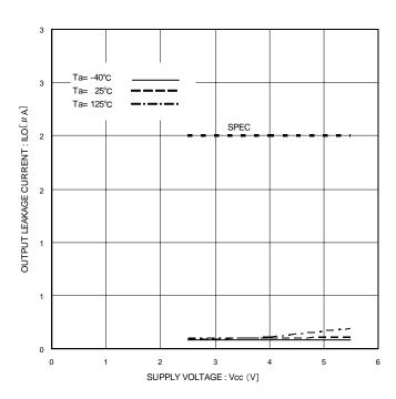
Figure 12. Output Leakage Current ILO(SO) (Vcc=5.5V)
