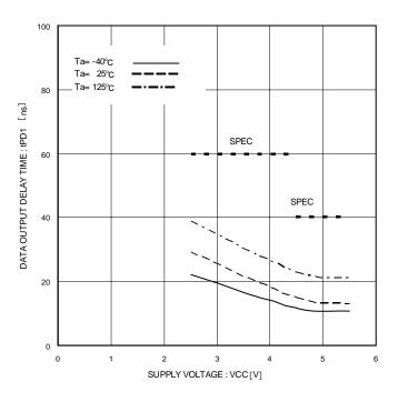
Figure 25. Data Output Delay Time tPD1 (CL=100pF)
