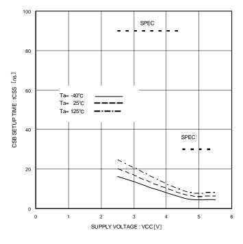
Figure 21. CSB Setup Time tCSS
