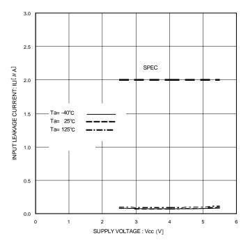
Figure 11. Input Leakage Current ILI (CSB,SCK,SI,HOLDB,WPB)
