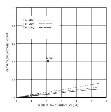
Figure 9. Output Low Voltage VOL, IOL (Vcc=2.5V)
