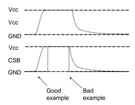
Figure 60. CSB timing at power ON/OFF
