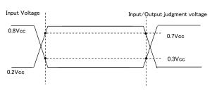
Figure 1. Input/Output judgment voltage
