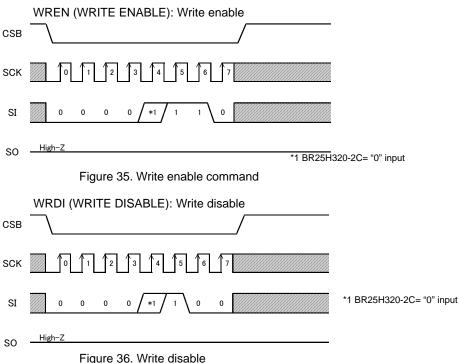
OThis IC has write enable status and write disable status. It is set to write enable status by write enable command, and it is set to write disable status by write disable command. As for these commands, set CSB LOW, and then input the respective ope codes. The respective commands accept command at the 7-th clock rise. Even with input over 7 clocks, command becomes valid.
