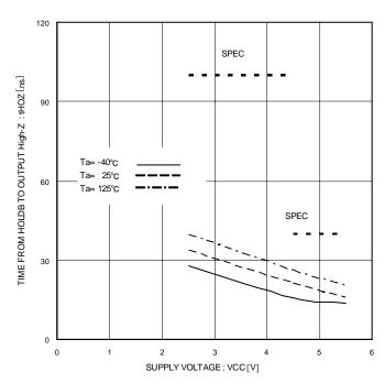
Figure 30. Time from HOLDB to Output High-Z tHOZ
