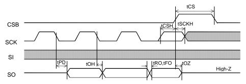
Figure 3. Input / Output timing
