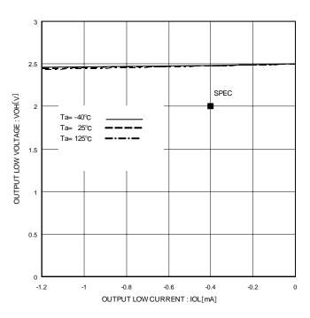
Figure 10. Output High Voltage VOH, IOH (Vcc=2.5V)
