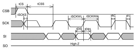
Figure 2. Input timing
