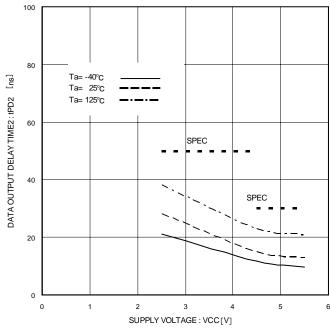
Figure 26. Data Output Delay Time tPD2 (CL=30pF)
