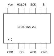
Figure 6. Pin assignment diagram
