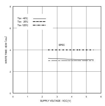
Figure 34. Write Cycle Time tE/W
