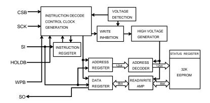
Figure 5. Block diagram
