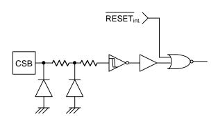
Figure 55. CSB input equivalent circuit
