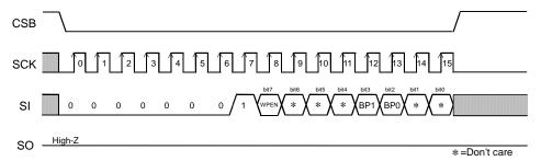
Figure 41. Status register write command
