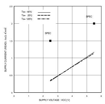
Figure 14. Supply Current (READ) ICC3,4
