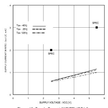
Figure 13. Supply Current (WRITE) ICC1,2
