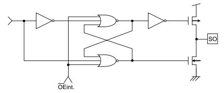
Figure 54. SO output equivalent circuit
