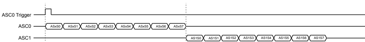
Figure 17-5. ASCx, ADCCTL.ADCMODE = 011b, 110b
