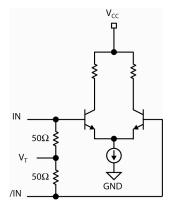
Figure 2. Simplified Differential Input Buffer
