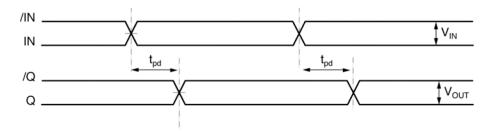
Figure 1a. Propagation Delay
