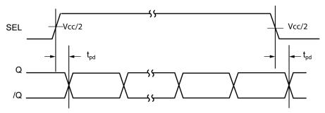
Figure 1c. SEL-to-Q Delay
