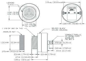
NOTE A: TERMINALS-032 BRASS TIN PLATED, TAPPED FOR #6-32 SCREW. TWO #6-32 NICKEL PLATED BRASS SCREWS INCLUBED. WILL ACCEPT 1/4' QUICK CONNECT. NOTE B: MOUNTING- REMOVE BLACK PLASTIC NUT
