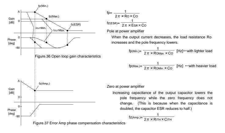
Stable feedback loop may be achieved by canceling the pole fp (Min.) produced by the output capacitor and the load resistance with CR zero correction by the error amplifier.
