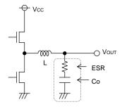
Figure.34 Output capacitor
