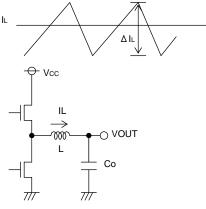
Figure.33 Output ripple current
