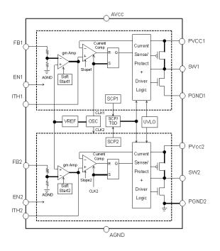
Figure.3 Block Diagram
