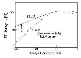
Figure.26 Efficiency characteristics
