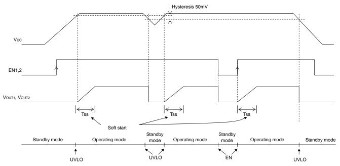
Figure.30 Soft start, Shut down, UVLO Timing chart
