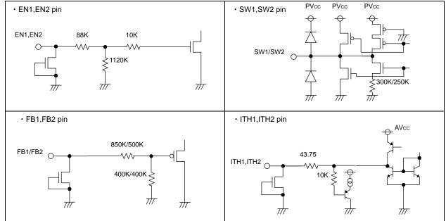
Figure.40 I/O equivalence circuit
