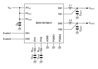
Figure.1 Typical Application Circuit
