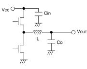
Figure.35 Input capacitor
