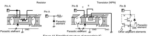
Figure.41 Simplified structure of monoclinic IC
