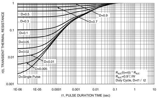
Figure 14. Transient Thermal Resistance
