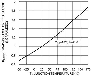
Figure 6. On-Resistance Variation with Junction Temperature
