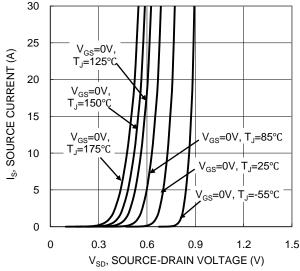
Figure 9. Diode Forward Voltage vs. Current
