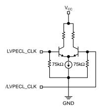
Figure 1. Simplified LVPECL Input Stage
