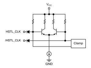
Figure 2. Simplified HSTL Input Stage
