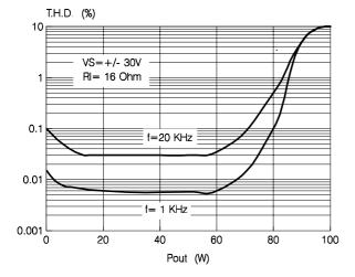
Figure 20: Distortion vs. Output Power
