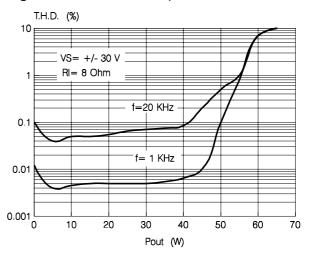
Figure 6: Distortion vs. Output Power
