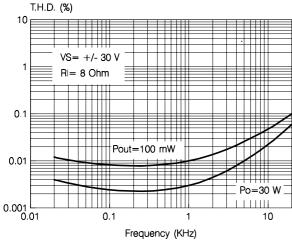
Figure 4: Distortion vs. Output Power
