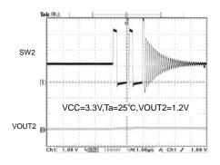
Fig.21 SW2 waveform (Io=0mA)
