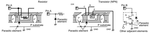
Fig.41 Simplified structure of monorisic IC
