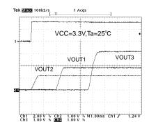
Fig.16 Soft start waveform (Io1=400mA,Io2=800mA,Io3=600mA)
