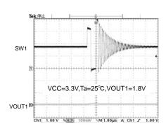
Fig.19 SW1 waveform (Io=0mA)
