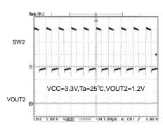
Fig.22 SW2 waveform (Io=800mA)
