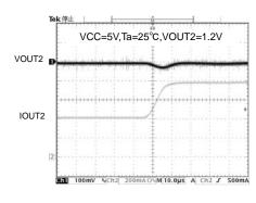
Fig.25 VOUT2 transient response (Io=400mA→800mA/ 10usec)
