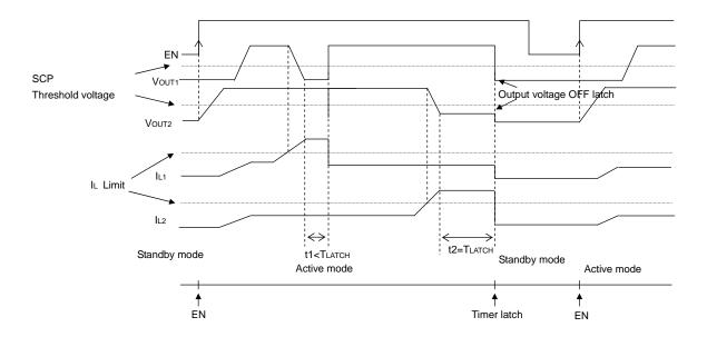
Fig.31 Timer latch short-current protection timing chart
