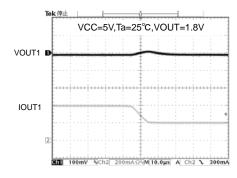
Fig.24 VOUT1 transient response (Io=400mA→200mA/ 10usec)
