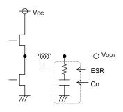
Fig.34 Output capacitor
