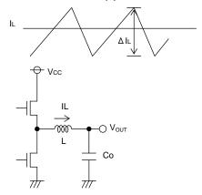
Fig.33 Output ripple current
