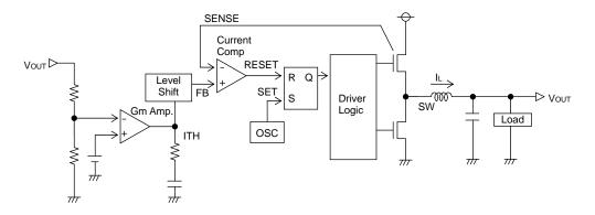
Fig.27 Diagram of current mode PWM control
