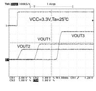
Fig.15 Soft start waveform (Io1=0mA,Io2=0mA,Io3=0mA)
