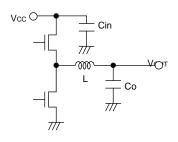
Fig.35 Input capacitor
