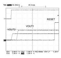
Fig.18 Soft start waveform (Io1=0mA,Io2=0mA,RESET)
