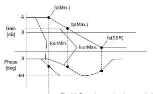
Fig.36 Open loop gain characteristics
