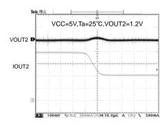
Fig.26 VOUT2 transient response (Io=800mA→400mA/ 10usec)
