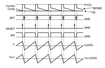
Fig.28 PWM switching timing chart
