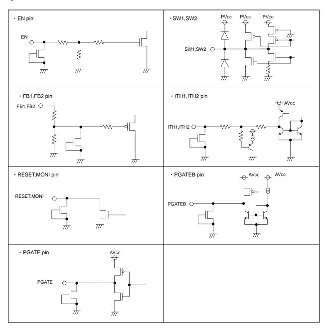
Fig.40 I/O Equivalent circuits
