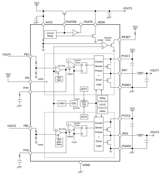
Fig.2 BD9151MUV Block Diagram
