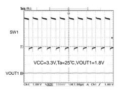
Fig.20 SW1 waveform (Io=400mA)
