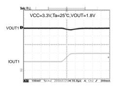
Fig.23 VOUT1 transient response (Io=200mA→400mA / 10usec)
