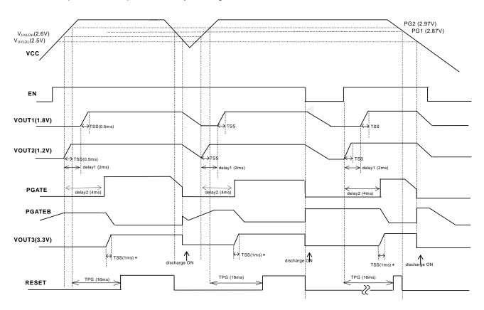
\*Starting time of VOUT3 TSS=1ms (when BD9151MUV is used) It depends on gate capacity when using Pch MOSFET
