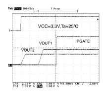
Fig.17 Soft start waveform (Io1=0mA,Io2=0mA,PGATE)
