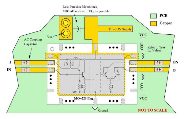
Biasing recommendations for positive supply with AC coupling applications
