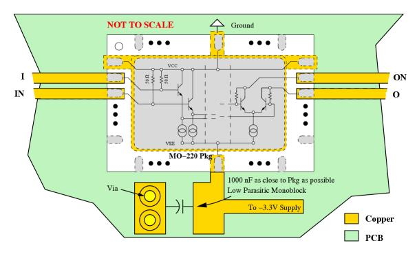
Biasing recommendations for negative supply with DC coupling applications
